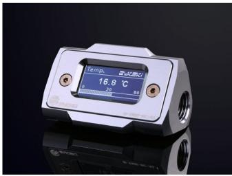
Users simply need to attach the sensors inline to the water cooling loop for instant water loop fluid temperature monitoring. The B-TME-SE-AL is designed for use on main loop tubing, and features an OLED display showing real-time temperature information. To read said temperature it uses a thermistor in the inlet screw, and temperatures are presented as either a progress bar or curve display. Construction is in aircraft-grade aluminium, and it comes in black and grey colours.
