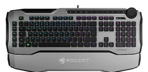
According to Roccat, membranical keys are more accurate in terms of actuation point compared to other rubber dome keys, allowing for fast yet silent (no clicking) typing. The keys are "mid-height," with an actuation speed of 7.8ms for the regular keys and 5ms for five low-profile macro keys. In addition, the keys sit in a laptop-style island layout to resist dirt.
