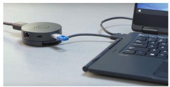
Described by the company as an ideal accessory for connecting multiple devices, including displays, printers and ethernet, the DA300 offers HDMI, VGA, DisplayPort, USB-A, USB-C and RJ45 ports. In turn it connects with PCs or laptops via retractable USB-C cable, and users can extend the cable by simply rotating the puck.
