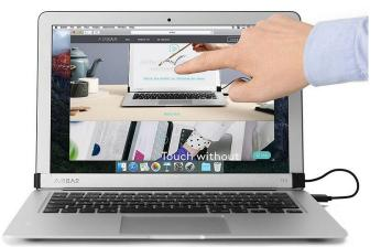
The AirBar is a slim aluminium bar one magnetically attaches to the bezel underneath the MacBook Air display. It plugs in via USB, and users may either immediately plug-and-touch or install multi-touch software, and it allows users to touch the screen with anything from a gloved finger to a paintbrush.
