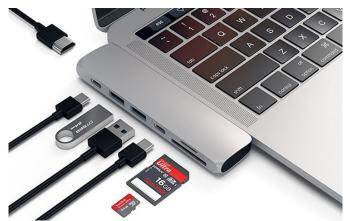
The Pro Hub is similar to the first <u>Satechi Type-C Hub</u>, but adds two Thunderbolt 3 dongles taking up both ports on either side of the latest MacBook Pro. Once plugged into the notebook the hub provides access to a passthrough Thunderbolt 3, USB-C port, HDMI and two USB 3.0 ports, as well as SD and microSD card readers.
