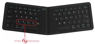
The keyboard features an ergonomic V-shape layout with a foldable and compact design, making it ideal for traveling customers. It uses Bluetooth 3.0 connectivity, is compatible with iOS, Android and Windows devices and carries a lithium-ion battery promising "hours" of typing on a single charge.
