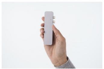
According to the company, the Hyperdrive uses the two USB-C ports on the MacBook Pro to deliver 45Gb/s bandwidth, thus allowing to simultaneous use of all 7 ports. This includes the connection of a 5K Thunderbolt 3 display or two 4K displays, as well as the delivery of up to 100W of power to charge the laptop at full speed.
