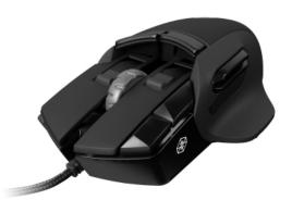
The above mentioned sensor array allows users to pivot, tilt and roll the mouse for an extra level of game control. For instance, the company suggests it as a means for flight simulator control by lifting and moving the mouse in the air, or tilting for crouch or lean controls in a shooter without need to press a keyboard button.
