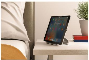
The Base supports both 12.9- and 9.7-inch versions of the iPad Pro. It features aluminium construction, a rubber anti-slip base, and the charging cradle uses magnets to align the device with the charging pins. Actual power comes through connecting a Lighting cable and power brick to the back of the Base.
