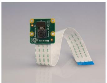
The original Pi camera board launched in 2013 and packed a 5MP OmniVision OV5647 sensor. Stocks of the sensor are "almost completely depleted," bringing about a need for an upgraded version. As such, the new camera accessory has a fixed-focus sensor capable of shooting 3280 x 2434 resolution still photos and 1080p video at 30fps.
