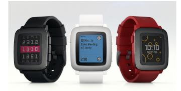
Like the first Pebble, the Pebble Time features four physical buttons and requires connection to a smartphone (via Bluetooth LE) for actual usability. However it replaces the monochrome ePaper display with a 64-colour version, while the stainless steel body is slimmer and slightly curved to hug the wrist better.
