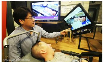
The EYECAN+ unit sits underneath the monitor, and does not require the user to sit in any specific position. Designed for use by the disabled, it only requires calibration for first-time users, and features a 2-mode UI in the shape of a rectangular menu board or wheel, each with 18 pre-configurable commands.
