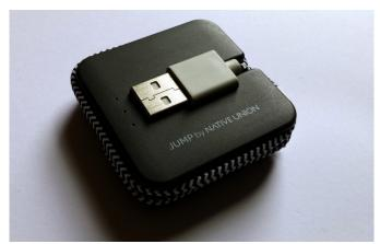
Native Union presents a novel take on the spare mobile device charger with the JUMP Cable-a charging cable with a built-in 800mAh battery providing faster charging and an extra bit of power.
