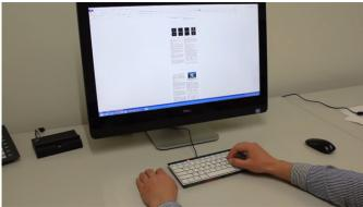
Dubbed "Type-Hover-Swipe in 96 Bytes", the prototype does not require users' fingers to be more than 1cm above the keyboard, meaning one can easily integrate gesture control with regular typing. This makes it more usable than the Leap Motion, which requires users to hover their hands around 30cm above the device.
