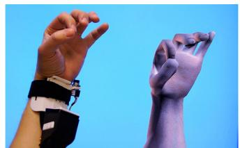
Dubbed the "Digits Project," the wrist-mounted device takes some inspiration from the Kinect. Using diffuse infrared light, IR laser, camera and inertial measurements the system software builds a 3D model of the moving hand the researchers claim is accurate to within one hundredth of a centimetre.
