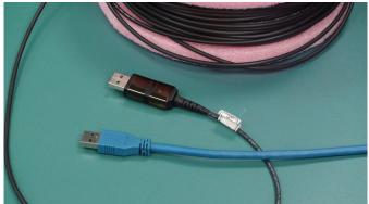
It features the VIA VO510 5-Gigagit optical transceiver (using light rather than electric signals), and is compliant with SuperSpeed USB electrical specifications. With an ultra-thin profile and long reach, the USB 3.0 AOC is ideal for of applications demanding rapid data transfer and HD multimedia capabilities.
