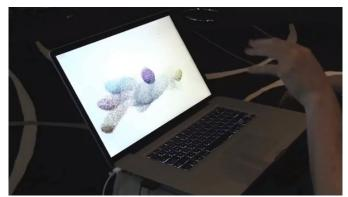
Connecting to PCs via USB, the Leap simultaneously tracks 10 fingers (or objects like a pen) within a 0.1 cubic-metre virtual workspace through the combination of industry-standard cameras and sensors and Leap Motion software.
