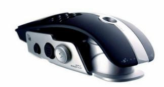
It features a skeletal design and an alumium base, with an LED-illuminated perforated midsection (supposedly to allow for airflow). The design is also customisable-- the rear is height-adjustable by 5mm and tiltable to either side by 5 degrees.
